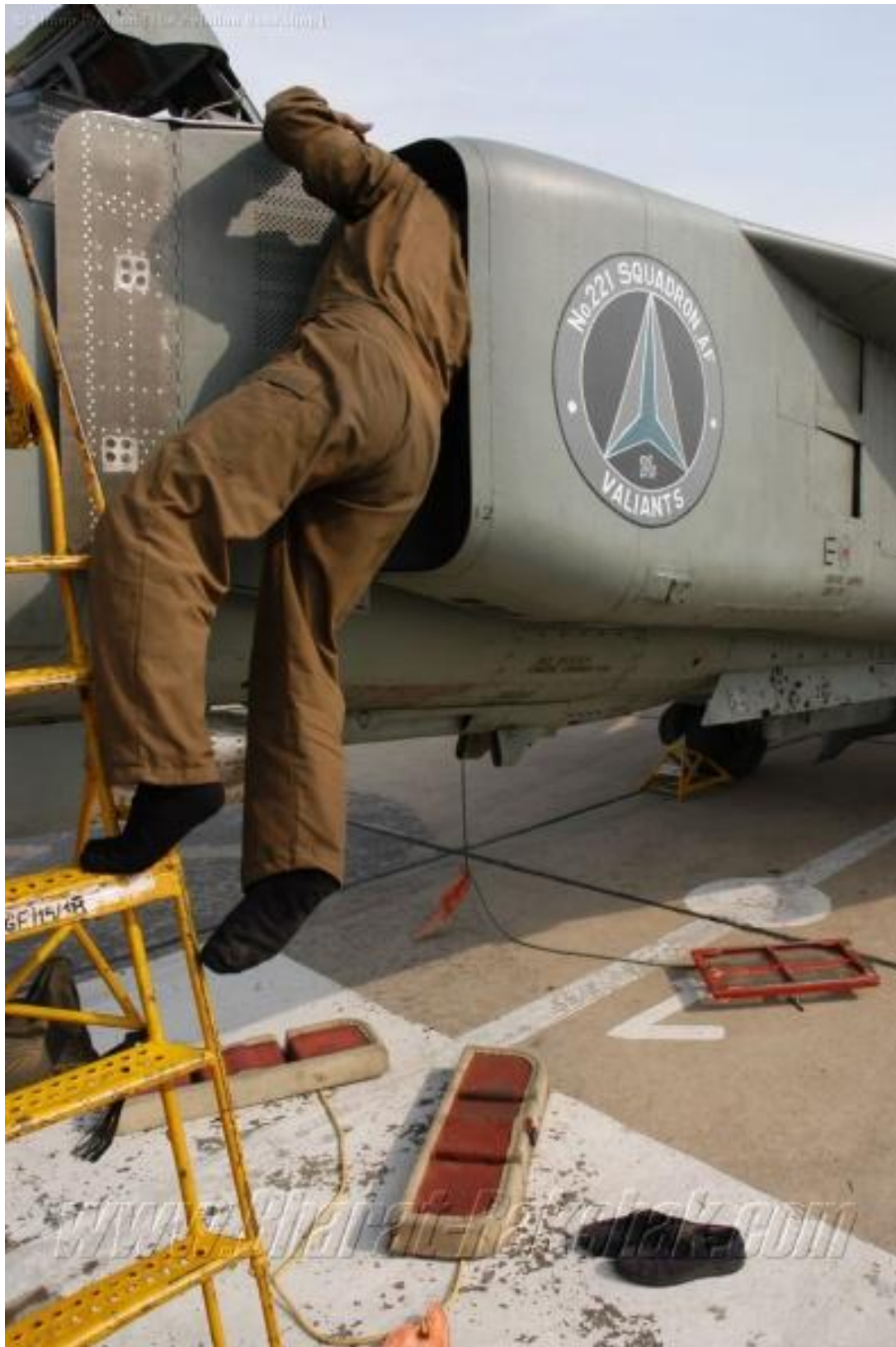
Image: A ground technician inspects a MiG-23BN at Halwara. Inspecting the engine by crawling into the intake requires both physical agility and technical expertise, which is not easy to achieve.
