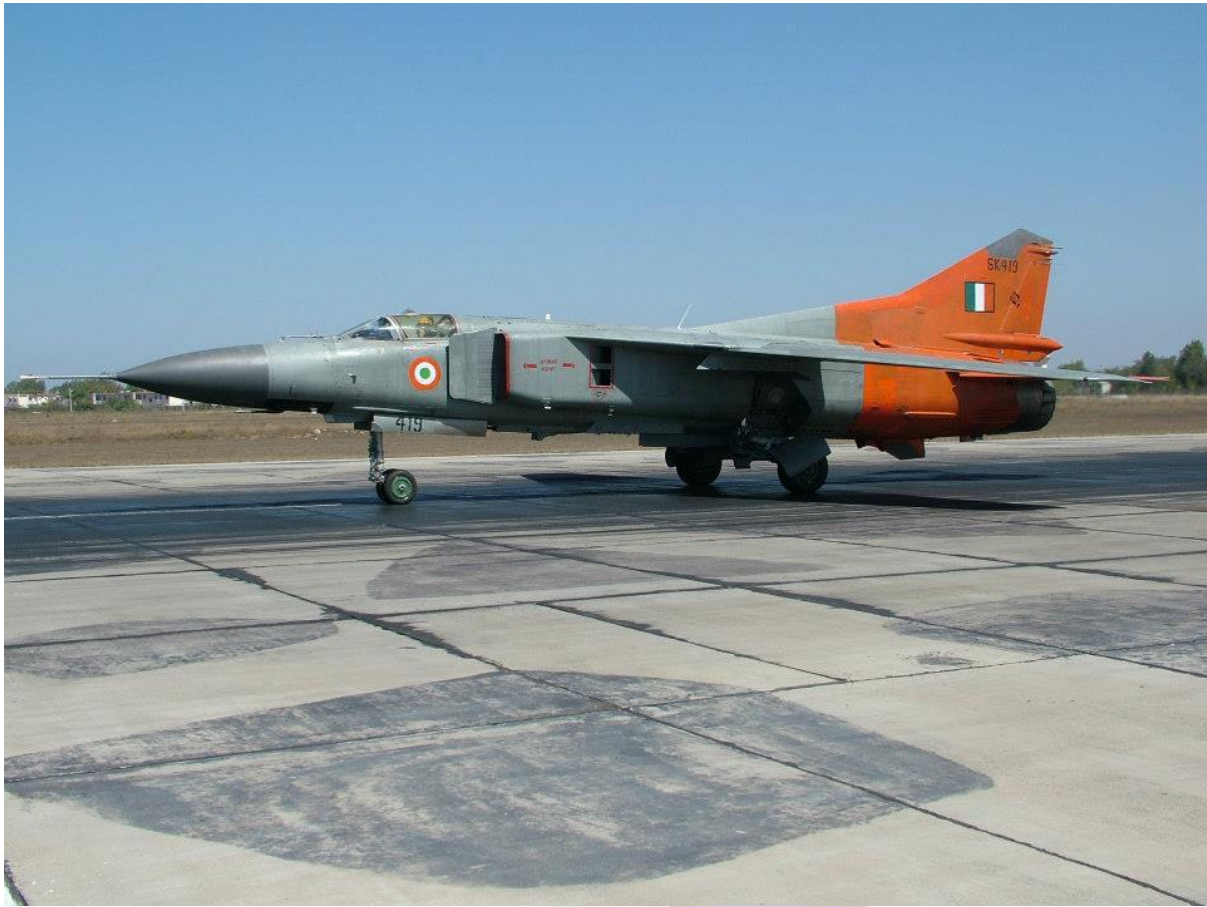
Image 8: MiG-23MF SK419 taken at Jamnagar sometime in 2005-06. This airframe is one of the six known MiG-23MFs to have been modified for Banner Target Towing, as distinguished by the orange-glazed tail (to make the aircraft much easier to spot) and the ventral fin removed to accommodate the tow-line. BTT duties were carried out over the air-air firing range near Kathiawar, situated in southern Gujarat.
