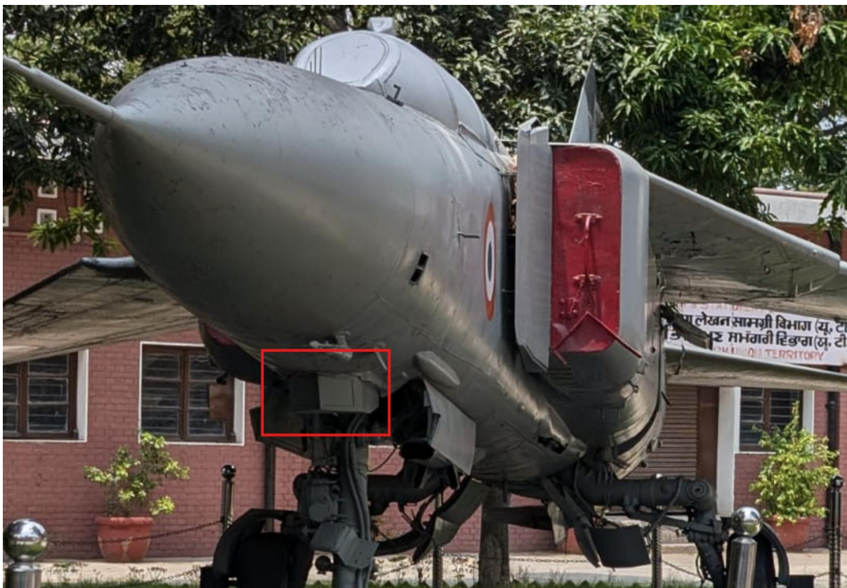
Image 4: An Indian Air Force MiG-23MF with the TP-23 IRST under the chin sensor marked.
