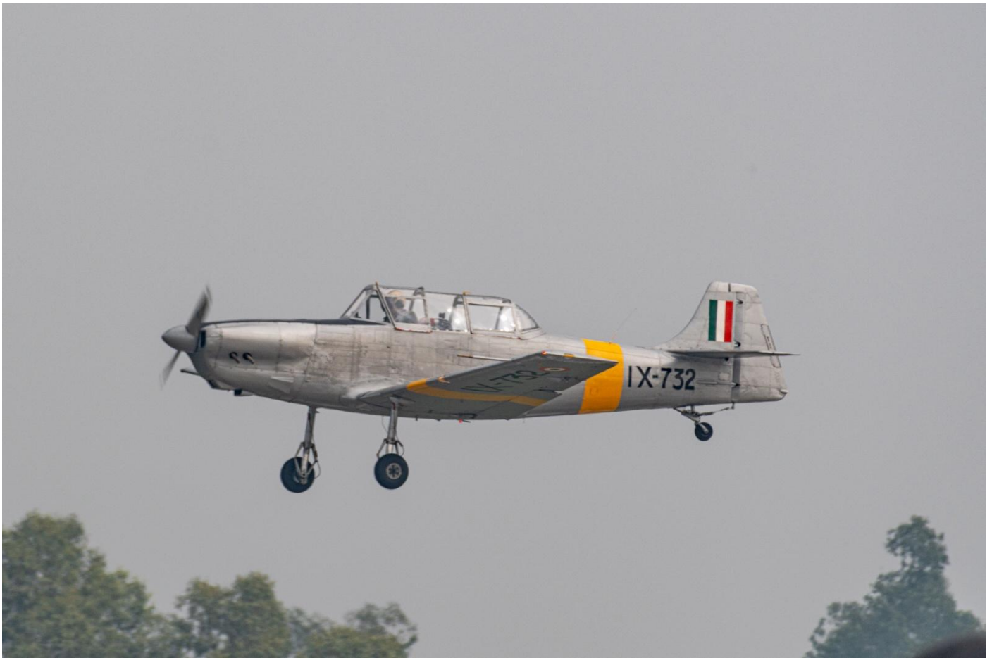
Caption: Inducted in 1955 as the air force's new basic trainer, the HT-2 was India's first indigenously designed and developed aircraft and manufactured by Hindustan Aeronautics Limited. Credit: Akshay Daniel
